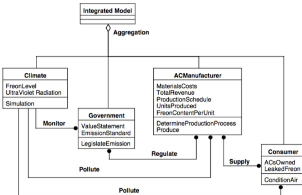
Figure 2: Integrated Model Object Diagram. Source: Jackson (1994)
